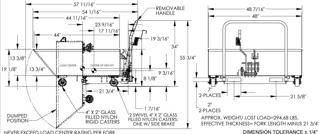
NEVER EXCEED LOAD CENTER RATING PER FORK TRUCK MANUFACTURER'S GUIDELINES. DO NOT USE THIS FORK TRUCK ATTACHMENT IF LOAD WILL EXCEED FORK TRUCK MANUFACTURER'S LOAD CENTER RATING.
